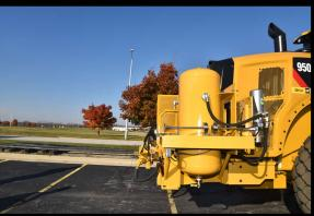
Cab controlled Power Alignment Railcar Coupler installed on a rubber tired Wheel Loader functions like a locomotive to move railcars. The railcar coupler and train brake hose folds up and pins in a lock position to provide the best possible machine approach and depart angles.
